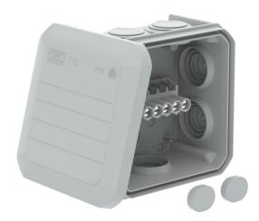
Junction box with terminal strip for the connection of cables and lines indoors and in protected outdoor areas. Square design with plug-in seals to the sides and knock-out entries in the bottom. Suitable for wall and ceiling mounting and on mounting panels. With the option to fasten inside. With fixed clamping cover. Made from halogen-free, UV-resistant materials.
