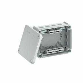
Junction box with terminal strip for the connection of cables and lines indoors and in protected outdoor areas. Rectangular design with plug-in seals to the sides and knock-out entries in the bottom. Suitable for wall and ceiling mounting and on mounting panels. With the option to fasten inside and to mount via the corner domes. Cover with quick lock, sealable. Made from halogen-free and UVresistant materials.
