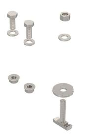
Screw set including hexagonal screws M12, hexagonal nuts with flange M12, hook-head bolt and washers. For the fastening of perforated straps, type LB FT, on rear supports on pre-assembled beams of PV open-field mounting systems.
