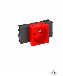
Earthing pin socket with connection to side, Single 0°, with increased touch protection, with screwless terminals, 2-pin, 16 A, 250 V~, with connection terminals to IEC 60884-1, suitable for the installation in Rapid 45 device installation trunking systems.
