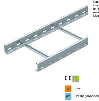
Cable ladder with 60 mm side height with riveted C profile rungs which are open in an upwards direction. Rolled side rail for reinforcement and as edge protection. Fastening to the bracket takes place using clamp, type LKS 40. The slot dimension of the frame is 11 mm and the appropriate U clamp is type 2056/N. Magnetic shield insulation without cover 10 dB, with cover 15 dB.
