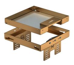
Height-adjustable cassette, decoupled from the floor, of nominal size 4, with cord outlet, for the installation of accessories in dry-cleaned floors indoors, for mounting in underfloor boxes UZD250 or UZD350, either in conjunction with a mounting cover DUG../4 or in UGD250-3/4 or UGD350-3/4. Mounting takes place using height-adjustment brackets (order separately) in the aluminium frame profile of the underfloor boxes.
