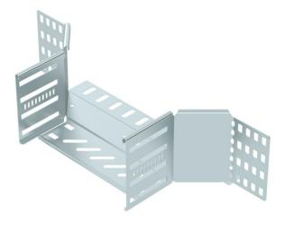
Add-on tee for the creation of a horizontal branch or cross-over, fitting for lock and screw-on cable trays of side height 110 mm. Screwless mounting with double clamps or screw connection with FRS truss-head screws and M6 combination nuts. Can be used in indoor areas. Fastening material must be ordered separately.
