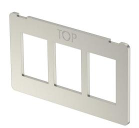
Support plate to accept three data connection modules of the following types: AMP TYCO: SL series 110Connect and Toolless, AMP-Twist; Brand-Rex: unshielded; GG45; TKM RJ MOD; Nexans: LANmark with Adapter Clip. Dimensions of a mounting opening in mm: 20.10 x 14.80.
