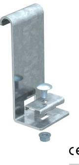
Connector for creation of branches at the same height at a later date. To increase the cable supporting surface, use a conjunction of corner plates of type LEB.
