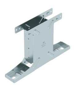
Base of the symmetrical floor support for the BKRS system, suitable for crossbeam type BSST 400/500/600. Can be used for walkable cable trays of width 400-600 mm. With threaded unions for mounting connection components, e.g. pipe clamps, as well as slots for floor mounting up to M10. Fastening material must be ordered separately.
