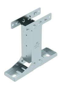
Base of the symmetrical floor support for the BKRS system, suitable for crossbeam type BSST 200/300. Can be used for walkable cable trays of width 200 or 300 mm. With threaded unions for mounting connection components, e.g. pipe clamps, as well as slots for floor mounting up to M10. Fastening material must be ordered separately.
