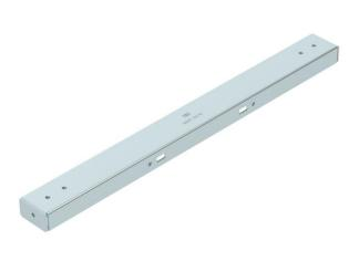
Crossbeam of the symmetrical floor support for the BKRS system, suitable for base type BSSU 190 4060. Can be used for walkable cable trays of width 500 mm. With threaded unions for cut-free mounting of cable trays. Fastening to base with 4x FKS M6 flat-head screws. Fastening material must be ordered separately.
