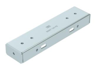
Crossbeam of the symmetrical floor support for the BKRS system, suitable for base type BSSU 190 2030. Can be used for walkable cable trays of width 200 mm. With threaded unions for cut-free mounting of cable trays. Fastening to base with 4x FKS M6 flat-head screws. Fastening material must be ordered separately.
