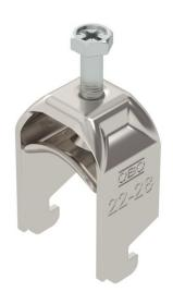
Clamp clip with N-foot, metal pressure sleeve with rounded edges to protect the cable. For vertical and horizontal mounting of 1 single cable on a C-profile rail. For slot width 11–12 mm With 1-start screw thread on pressure sleeve, universal hexagonal screw head WAF10, with slot and cross recess. Suitable for assembly indoors and outdoors. We recommend the use of a counter-sleeve.
