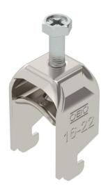
Clamp clip with N-foot, metal pressure sleeve with rounded edges to protect the cable. For vertical and horizontal mounting of 1 single cable on a C-profile rail. For slot width 11–12 mm With 1-start screw thread on pressure sleeve, universal hexagonal screw head WAF10, with slot and cross recess. Suitable for assembly indoors and outdoors. We recommend the use of a counter-sleeve.
